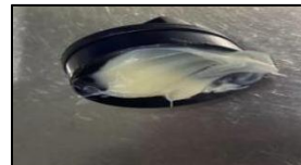
一字键槽内填充油脂 Fill the slotted keyway with grease
